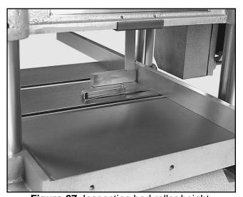
Figure 27. Inspecting bed roller height.
